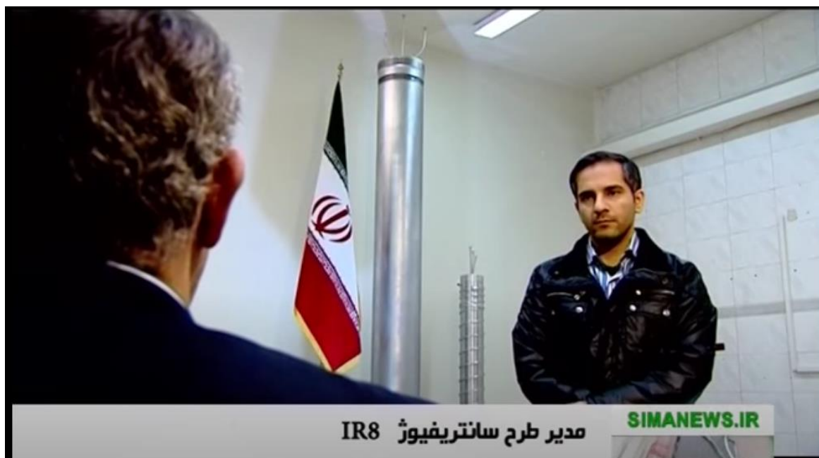
Figure 1.21. An IR-8 outer casing, with feed and withdrawal tubes on top, can be seen in the background, next to an unidentified centrifuge, possibly an IR-1. Source: Screen capture from Simanews.ir/IRIB
