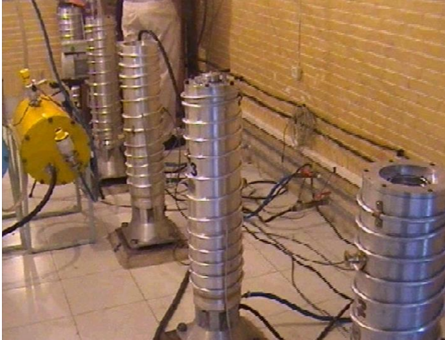
Figure 1.9. A photo, captured from an Iranian video in the Nuclear Archive, of individual centrifuge outer casings on stands in an unknown facility. The outer casings do not appear to contain centrifuge rotors.
