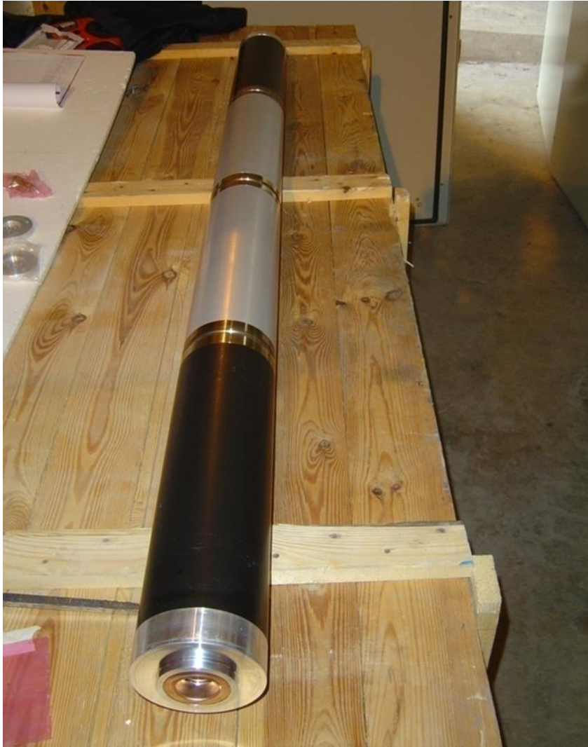
Figure 1.6. An IR-1 centrifuge rotor assembly, showing three bellows, four rotor tubes, and an end cap. The image was taken in Libya, where the rotor assembly was supplied by Pakistan.
