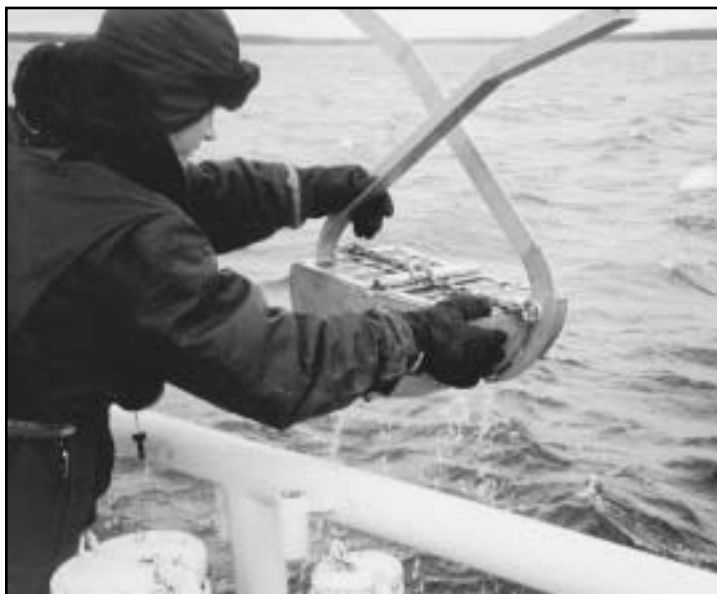
Water sampling: here IAEA inspectors are testing techniques to detect very small quantities of plutonium or other elements that would indicate the production of separated plutonium.
